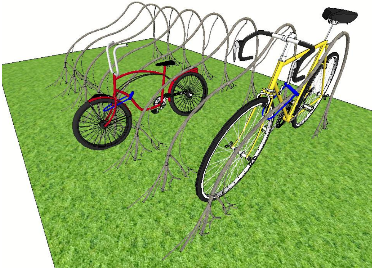
Figure 4) Rendering of vine-shaped bike rack design illustrated with an adult and a child bicycle, both with standard u-locks. The sloped shape of the vine allows any size bicycle to be locked with a standard u-lock. Cross-bracing “vines” are designed to not interfere with the bicycle rear tire.
